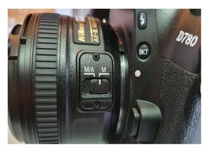
16. Set the AF Switch on the camera to 'M'
