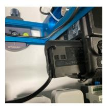
20. Use one of the USB connections inside the RSC LED (position 5, page 9) to connect the rectangular USB cable to the LED controller.
