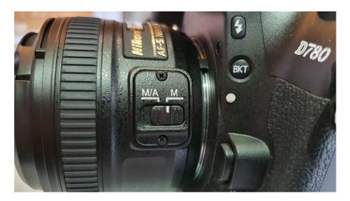
13. Set the AF Switch on the camera to 'M'
