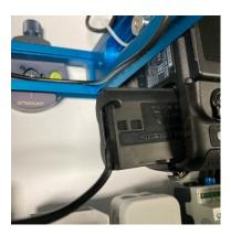
17. Use one of the USB connections inside the RSC LED (position 5, page 9) to connect the rectangular USB cable to the LED controller.
