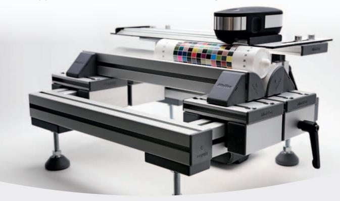
The Measure Mount is a device for the use of the i1Basic Pro 2 hand-held measuring device from X-Rite for the color measurement of cylindrical shaped and hollow bodies such as cans, bottles, tubes and glasses.
