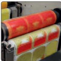
Flexo printing is often used in the packaging printing sector. It is common practice to print on non-absorbing substrates by using screen rulings between 60 lpi up to 150 lpi with partially high increase in dot gains.
